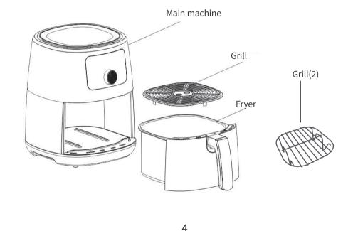
Product Structure and Features Before use 1.Remove all packaging materials, stickers, and labels 2.Clean the grill and pan with hot water, soap and no 3.Wipe the inside and outside of the device with clean Note: Because the device operates in hot air, it is not oil and air frying oil. How to Use Your Airfryer The airfryer has a knob to select among functions an
